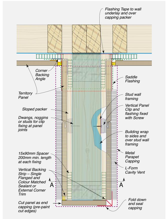
FIGURE 8.25 Two Sided Parapet – Elevation A
