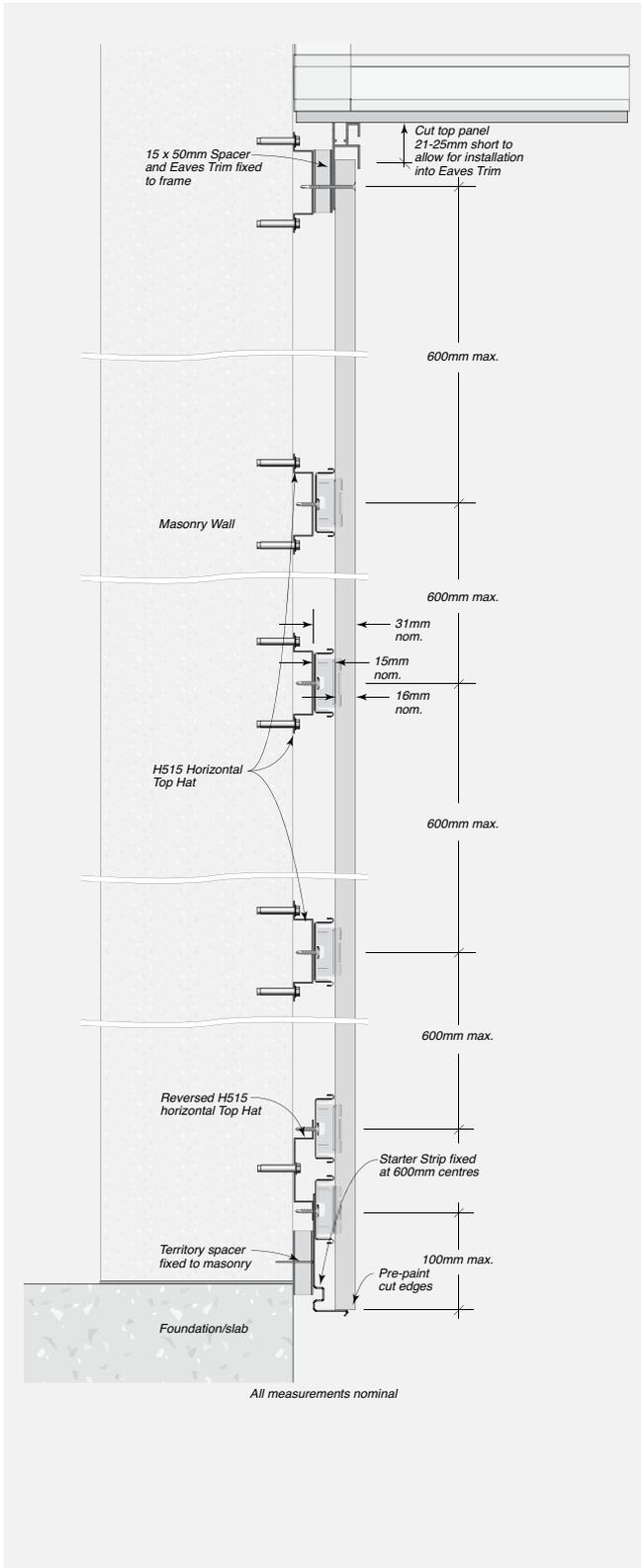
**FIGURE 7.14** Typical Face Fastening at Square Edge Joint - Elevation
