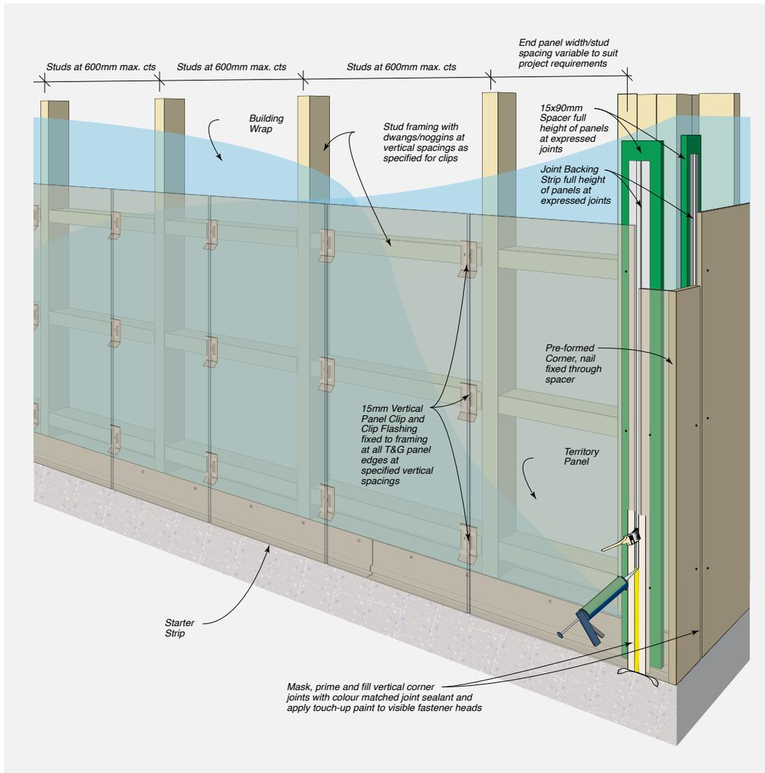
Designer Series clips, together with spacer strips, base starter strips and head vents/eaves trims, create a 15mm cavity behind the Territory panels which allows air flow, ventilation and drainage. This prevents moisture build up and reduces the risk of moisture penetration, allowing the building shell to dry out, creating a healthier, more breathable building.
