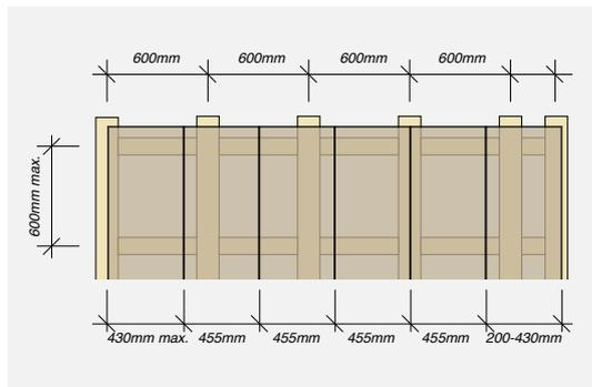
**FIGURE 7.02** Symmetrical Panel Set-out – Timber Framing
