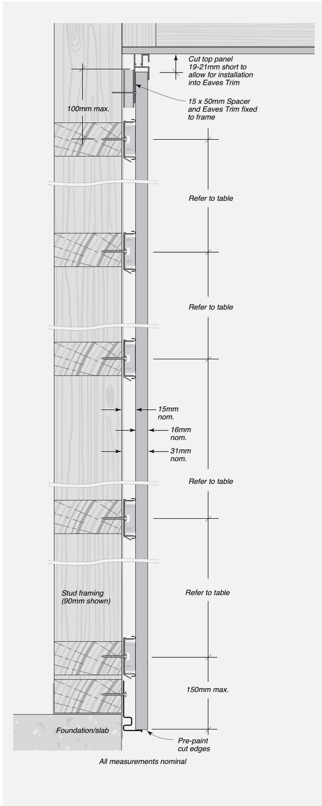
FIGURE 7.07 Typical Face Nailing at Square Edge Joint - Elevation
