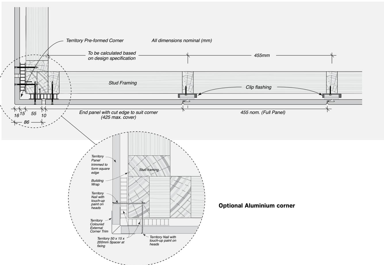
FIGURE 7.06 Typical Territory System Cross Section - Elevation
