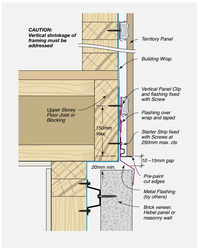
**FIGURE 8.04** Second Storey Junction with Masonry, Brick Veneer or Hebel Panels - In-line Framing
