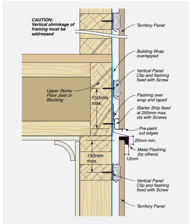
**FIGURE 8.19** Horizontal Control Joint – Between Panels
