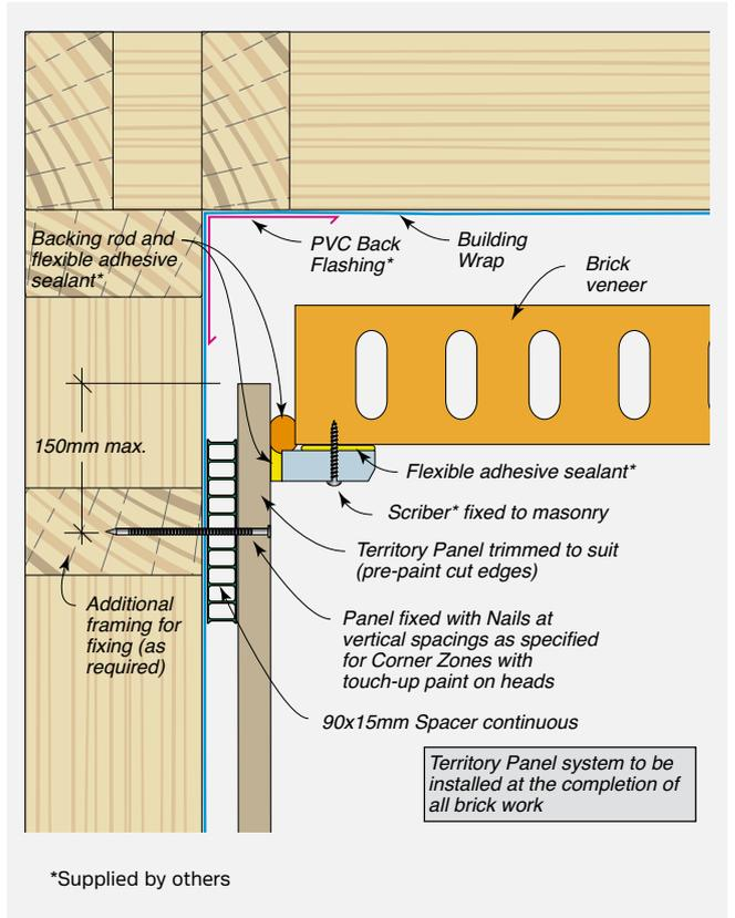
**FIGURE 8.30** Typical Abutment – Panel to Brick Veneer – Plan View
