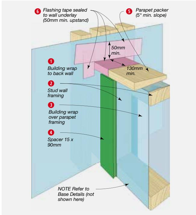
**FIGURE 8.28** Two Sided Parapet Wall Junction – Stage 3 Procedure
