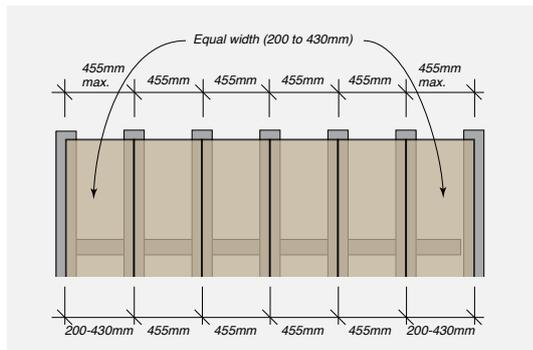
Note: For framing other than 455mm centres, horizontal structure members can be used (eg. top hats and additional timber framing). Contact DesignLink for further information.
