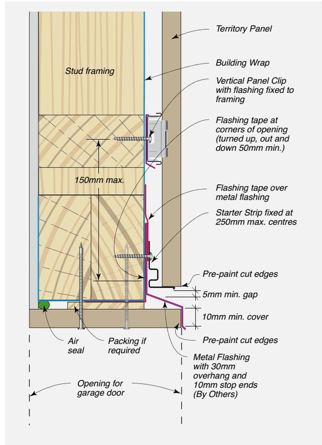
**FIGURE 8.16** Typical Penetration
