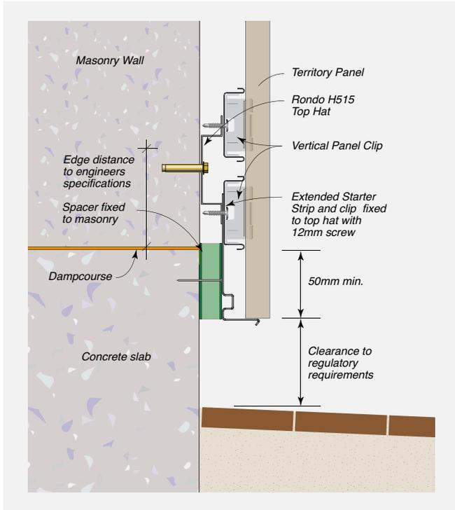
**FIGURE 8.41** Horizontal Control Joint – Second Storey Junction – Open Cavity
