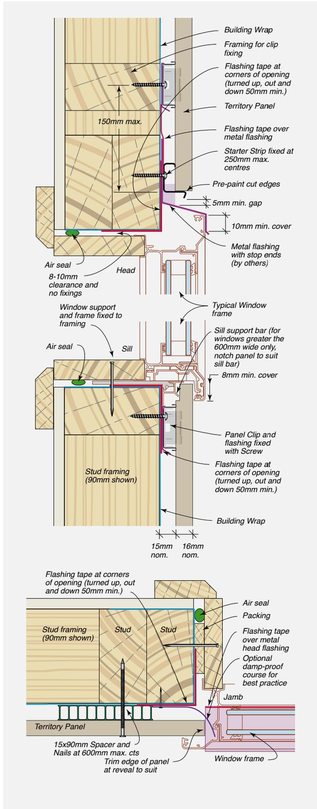
**FIGURE 8.13** Typical Window Head/Jamb Detail –Front Elevation
