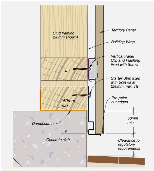
**FIGURE 8.03** Base Detail - Beam & Joist Construction
