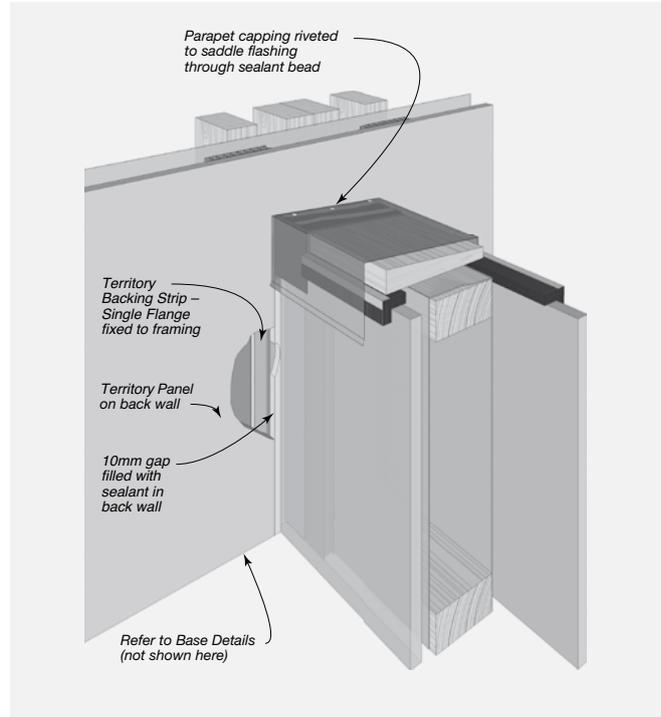
**FIGURE 8.27** Two Sided Parapet Wall Junction – Stage 2 Procedure
