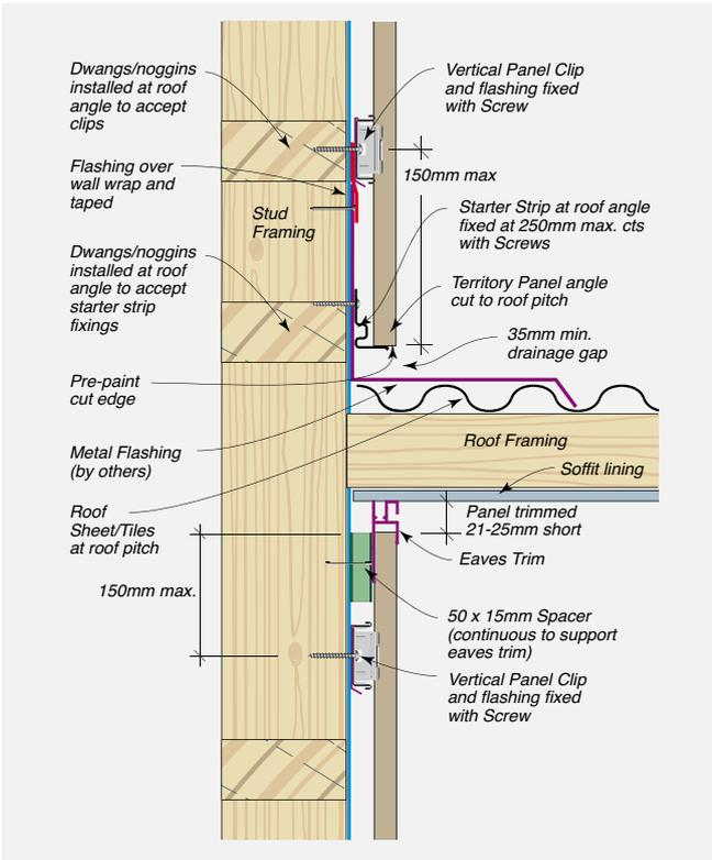
FIGURE 8.23 Junction of with External Roofing
