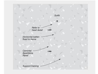
The junction between the wall and soffit can lead to wind and moisture ingress issues that need to be managed. A soffit junction typically means a discontinuation in the wall; therefore, you need to allow any unforeseen trapped moisture in the cavity to freely drain out as well as diverting moisture from travelling down the façade. The above wall to soffit detail provides one suggestion.
