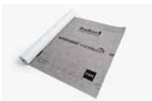
**Enviroseal™ ProctorWrap™ CW** is a light duty, triple layer spun bond vapour permeable wall wrap with a heavier weight protective fabric than ProctorWrap™ RW. It is tough, yet light, making it easy to handle during installation and is printed with a 150mm lap line to make alignment of overlaps simple.
